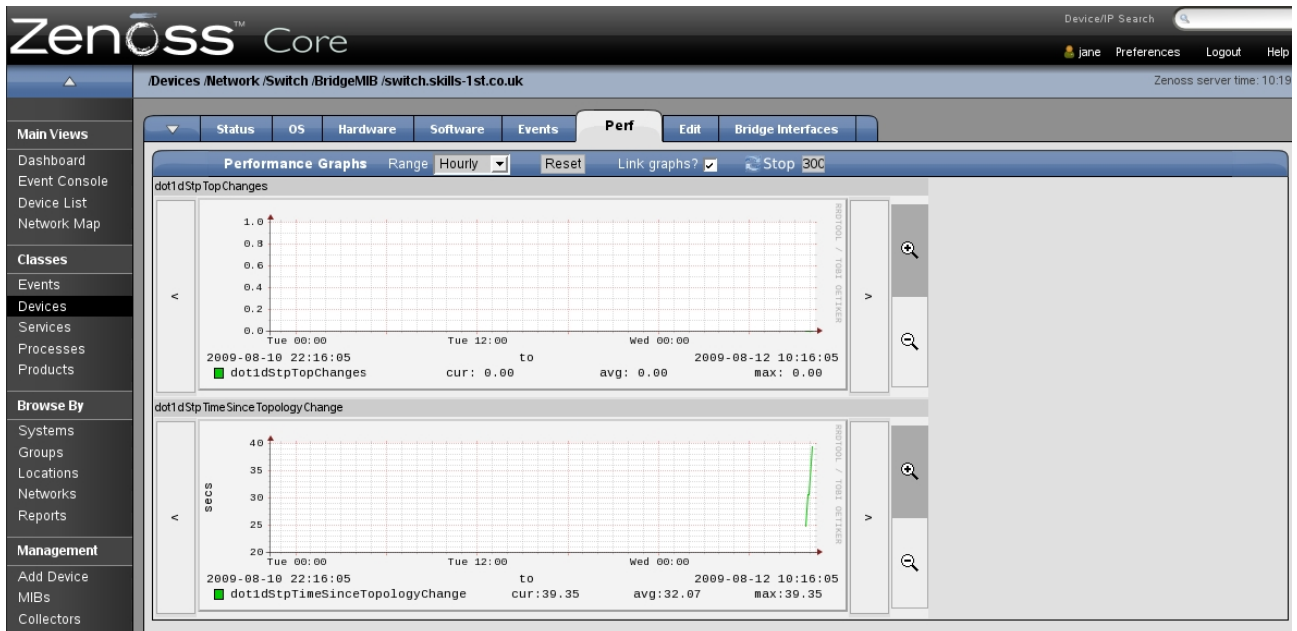
Figure 60: Performance graph for switch showing dot1dStp data
