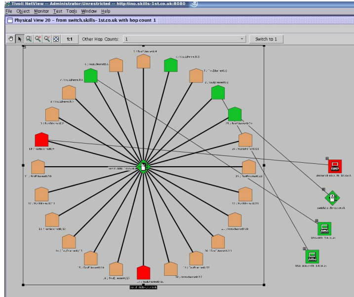
Figure 17 switch with 2 ports in Layer 2 fault condition
