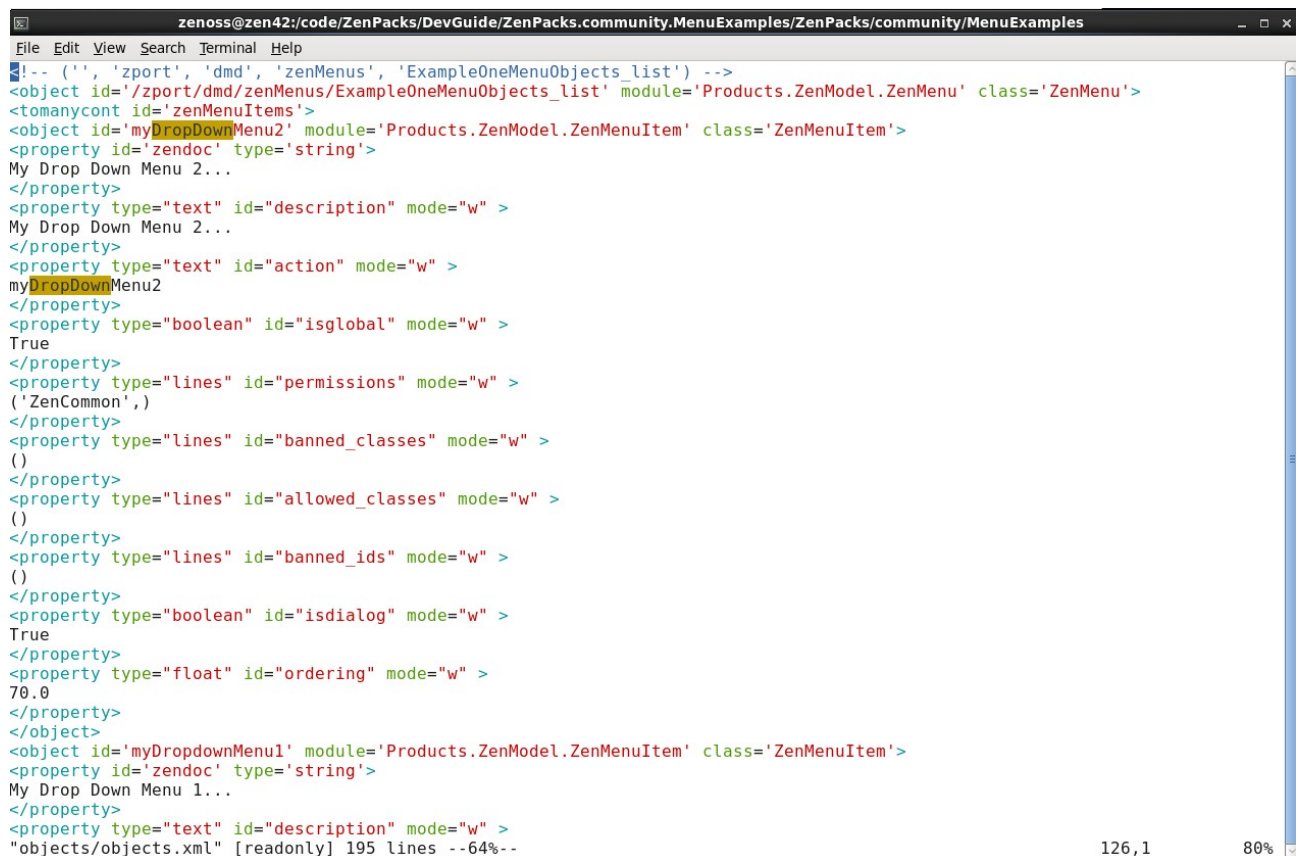
Figure 223: Definition of a menu list and its menus in objects.xml
