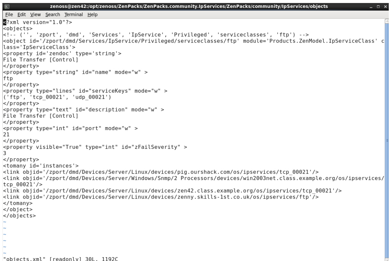
Figure 20: objects.xml for ZenPacks.community.IpServices - note entry for instances
